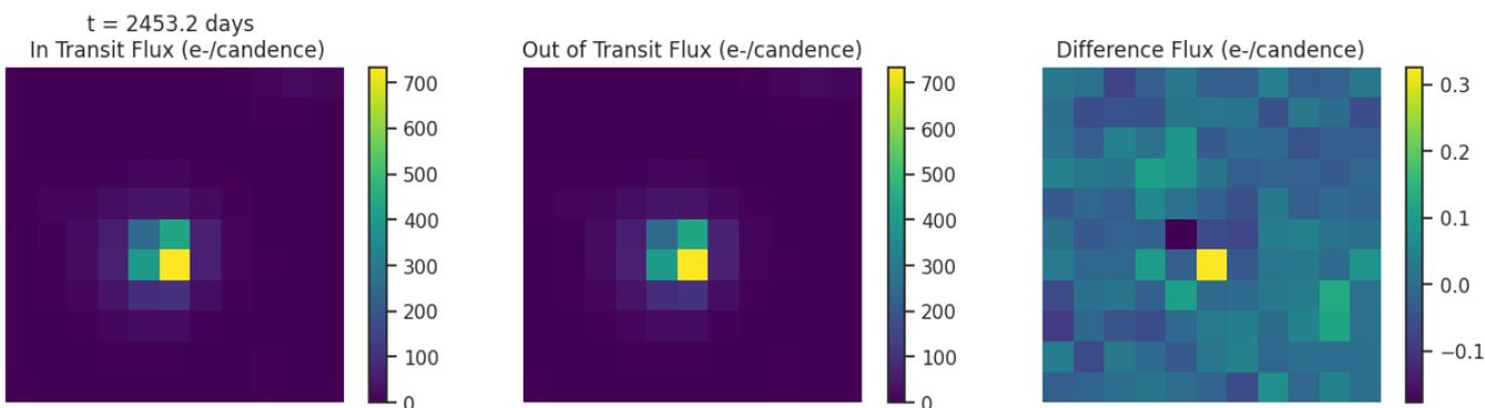
Fig 6. Difference images for target TIC 269848053 for each transit like event. Left: mean in-transit flux(left). Middle: mean out-of-transit flux. Right: difference between the mean out-of-transit and mean in-transit flux. Ensure that the change in brightness occurs on target.
