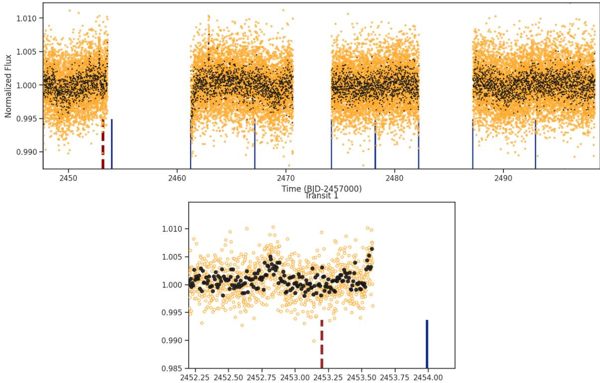
Fig 1. Full lightcurve for target TIC 269848053. The solid blue lines at the bottom of the figure indicated the times of the reaction wheel momentum dumps and the dashed black line(s) show the time(s) of the marked transit event(s). Momentum dumps occur around every 2 to 2.5 days and typically last around half an hour.
