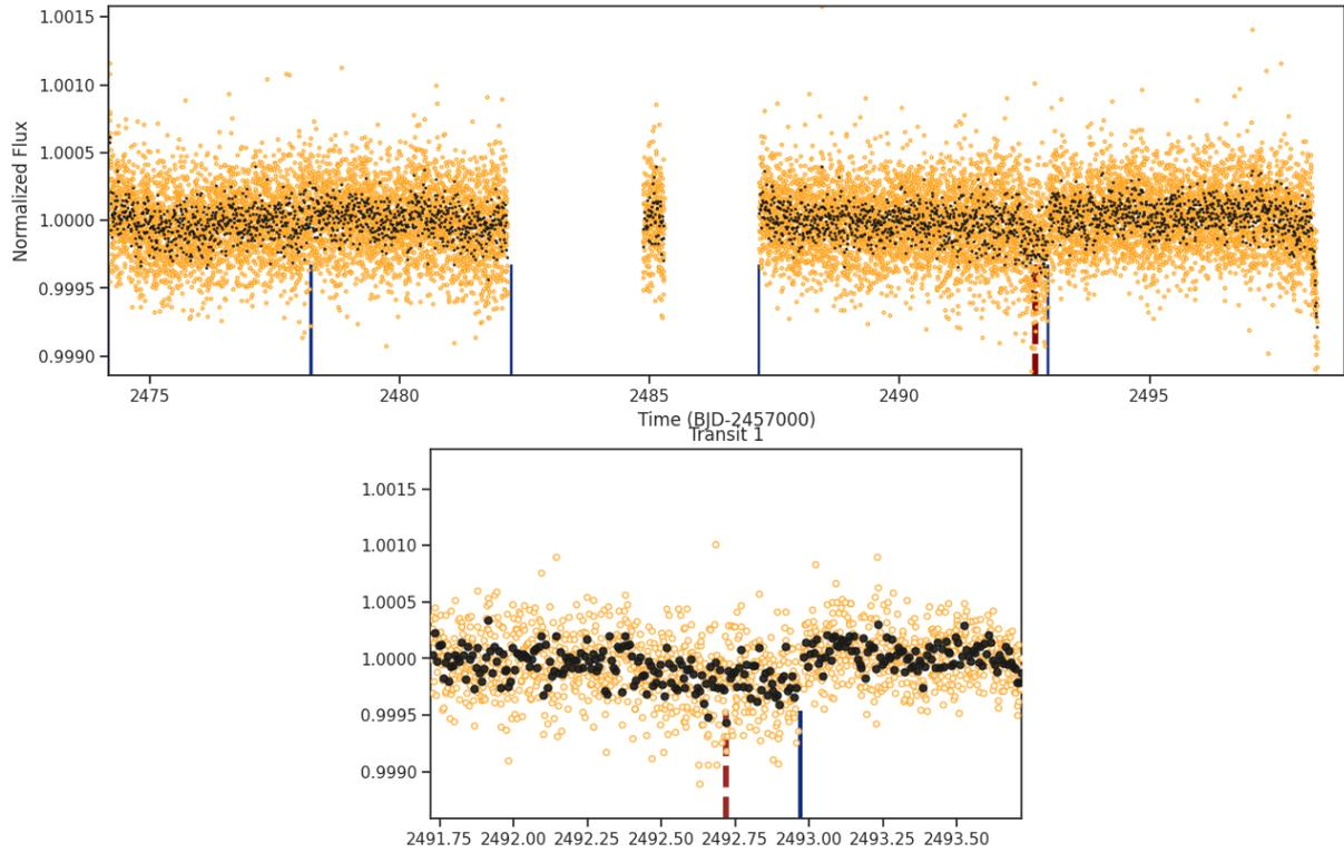
Fig 1. Full lightcurve for target TIC 262809788. The solid blue lines at the bottom of the figure indicated the times of the reaction wheel momentum dumps and the dashed black line(s) show the time(s) of the marked transit event(s). Momentum dumps occur around every 2 to 2.5 days and typically last around half an hour.
