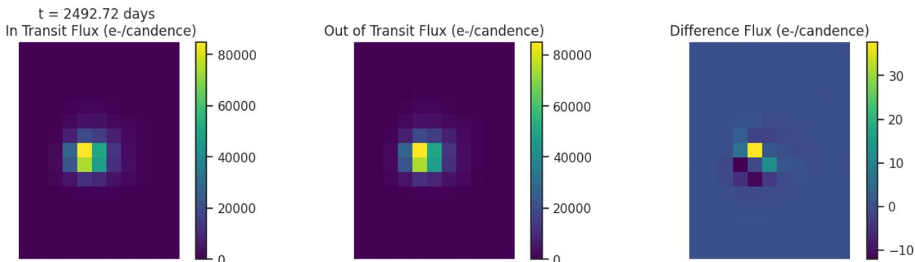
Fig 6. Difference images for target TIC 262809788 for each transit like event. Left: mean in-transit flux(left). Middle: mean out-of-transit flux. Right: difference between the mean out-of-transit and mean in-transit flux. Ensure that the change in brightness occurs on target.
